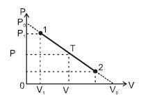
where  $\Delta U$  is the change in the internal energy of the gas; and W is work, done by the gas. For one mole of the monatomic ideal gas  $\Delta U = 3/2R$   $\Delta T$ . Work equals the area under the graph P vs. V
