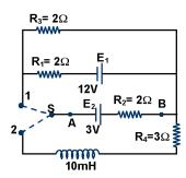
**Sol.** (a) When the switch is in position 1, the equivalent circuit is shown in the figure. No current flows through the inductor.
