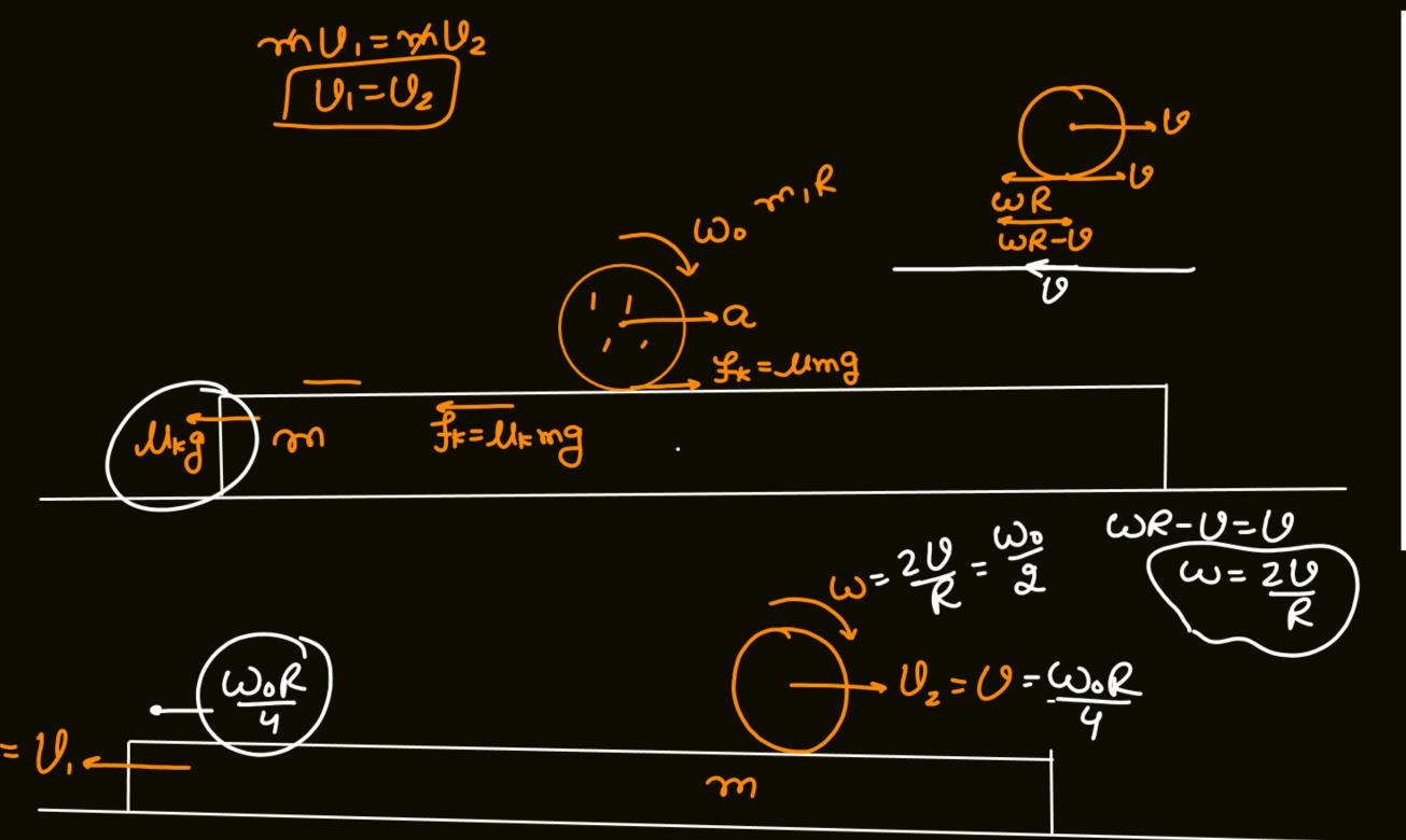
In the figure shown a plank of mass m is lying at rest on a smooth horizontal surface. A cylinder of same mass m and radius r is rotated to an angular speed  $w_0$  and then gently placed on the plank. It is found that by the time the slipping between the plank and the cylinder cease, 50% of total kinetic energy of the cylinder and plank system is lost. Assume that plank is long enough and  $\mu$  is the coefficient of friction between the cylinder and the plank.
