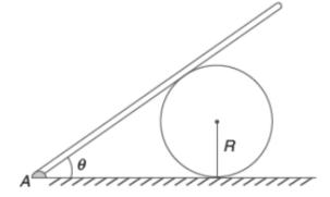
A ring of mass M and radius R is held at rest on a rough horizontal surface. A rod of mass M and length  $L=2\sqrt{3}R$  is pivoted at its end A on the horizontal surface and is supported by the ring. There is no friction between the ring and the rod. The ring is released from this position. Find the acceleration of the ring immediately after the release if  $\theta=60^{\circ}$ . Assume that friction between the ring on the horizontal surface is large enough to prevent slipping of the ring.
