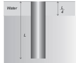
The upper liquid is water and the lower liquid has density twice that of water. The two liquid are immiscible. The cylinder is in equilibrium with its  $\frac{3}{4}$  length in the denser liquid and  $\frac{1}{4}$  of its length in water. The thickness of water layer is  $\frac{L}{4}$  only.
