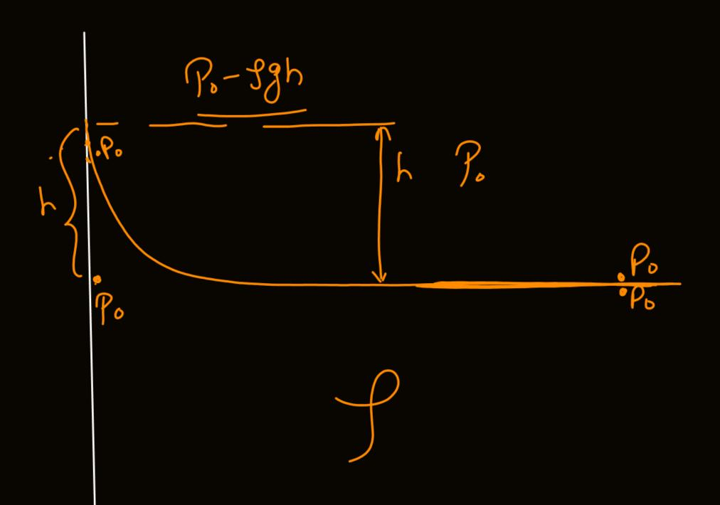
A liquid having surface tension T and density  $\rho$  is in contact with a vertical solid wall. The liquid surface gets curved as shown in the figure. At the bottom the liquid surface is flat.
