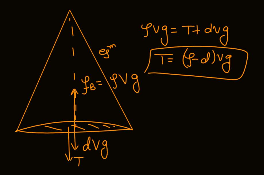
A solid wooden cone has been supported by a string inside water as shown in the figure. The radius of the circular base of the cone is R and the volume of the cone is V. In equilibrium the base of the cone is at a depth H below the water surface. Density of wood is d ( $< \rho$ , density of water).
