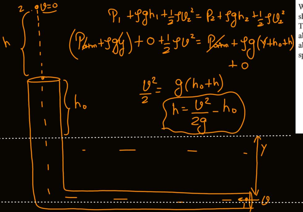
Water is flowing in a stream at speed v. A L shaped tube is lowered into the stream as shown. The upper end of the tube is held at a height  $h_0$  above the surface of the water. To what height 'h' above the upper end of the tube, will the water jet spurt? Assume that flow remains ideal.
