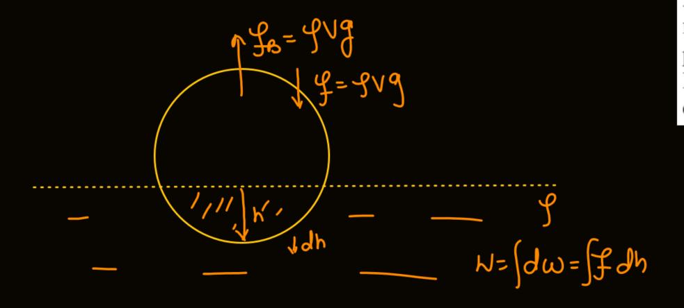
A sphere of radius R and having negligible mass is floating in a large lake. An external agent slowly pushes the sphere so as to submerge it completely. How much work was done by the agent? Density of water is  $\rho$ .
