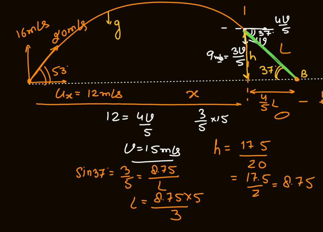
AB is a pipe fixed to the ground at an inclination of 37°. A ball is projected from point O at a speed of u = 20m/s at an angle of 53° to the horizontal and it smoothly enters into the pipe with its velocity parallel to the axis of the pipe. [Take  $g = 10 \text{ ms}^{-2}$ ]
