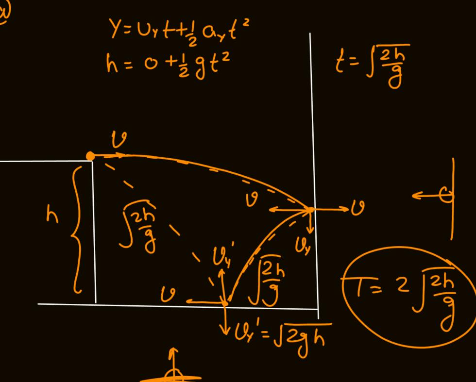
(a) A particle is thrown from a height h horizontally towards a vertical wall with a speed v as shown in the figure. If the particle returns to the point of projection after suffering two elastic collisions, one with the wall and another with the ground, find the total time of flight. [Elastic collision means the velocity component perpendicular to the surface gets reversed during collision.]
