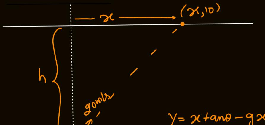
A horizontal electric wire is stretched at a height h = 10 m above the ground. A boy standing on the ground can throw a stone at a speed  $u = 20 ms^{-1}$ . Find the maximum horizontal distance x at which a bird sitting on the wire can be hit by the stone.
