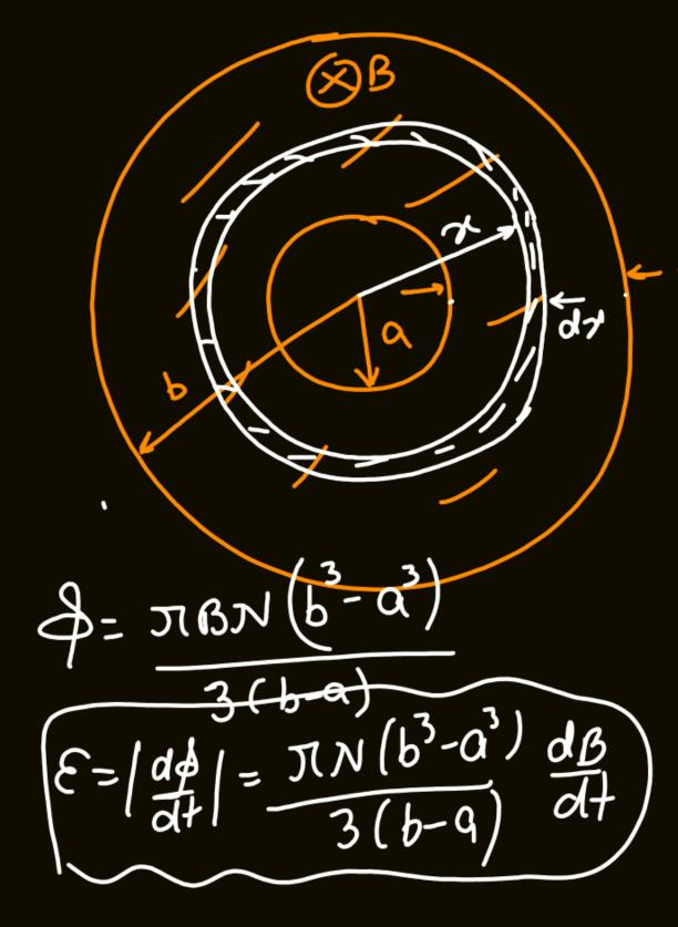
Q. 14: A flat coil, in the shape of a spiral, has a large number of turns N. The turns are wound tightly and the inner and outer radii of the coil are a and b respectively. A uniform external magnetic field (B) is applied perpendicular to the plane of the coil. Find the emf induced in the coil when the field is made to change at a rate  $\frac{dB}{dt}$ .
