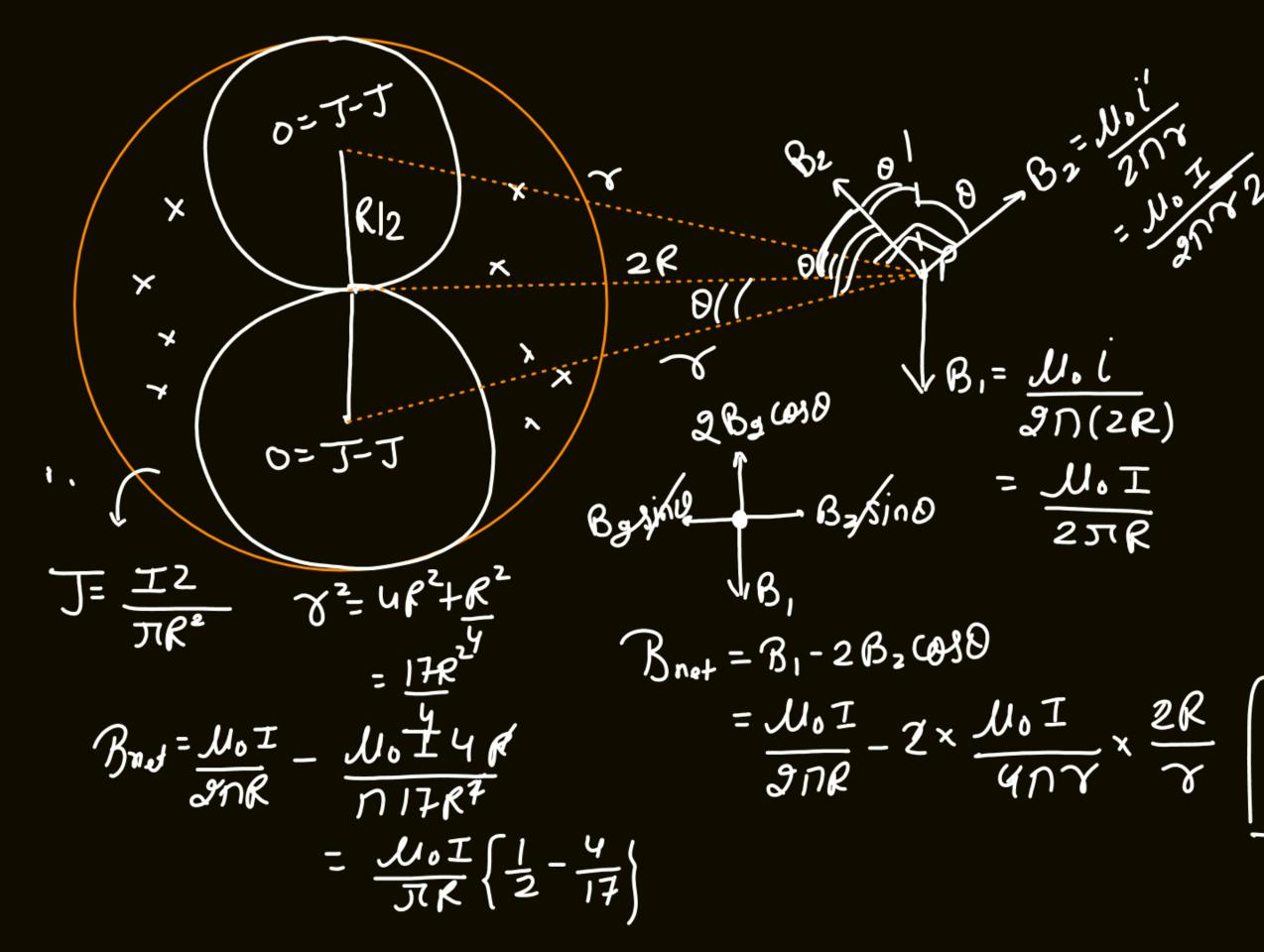
Q. 14: A long cylindrical conductor of radius R has two cylindrical cavities of diameter R through its entire length, as shown in the figure. There is a current I through the conductor distributed uniformly in its entire cross section (apart from the cavity region). Find magnetic field at point P at a distance r = 2R from the axis of the conductor (see figure).
