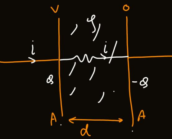
**Q. 44:** A parallel plate capacitor has plate area A and separation between the plates equal to d. A material of dielectric constant K and resistivity  $\rho$  is filled between the plates. The switch is closed to connect the capacitor to a cell of emf V.
