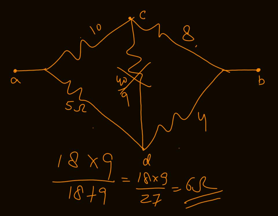
**Q. 10:** Find the equivalent resistance between point *a* and *b* in the network shown in figure.
