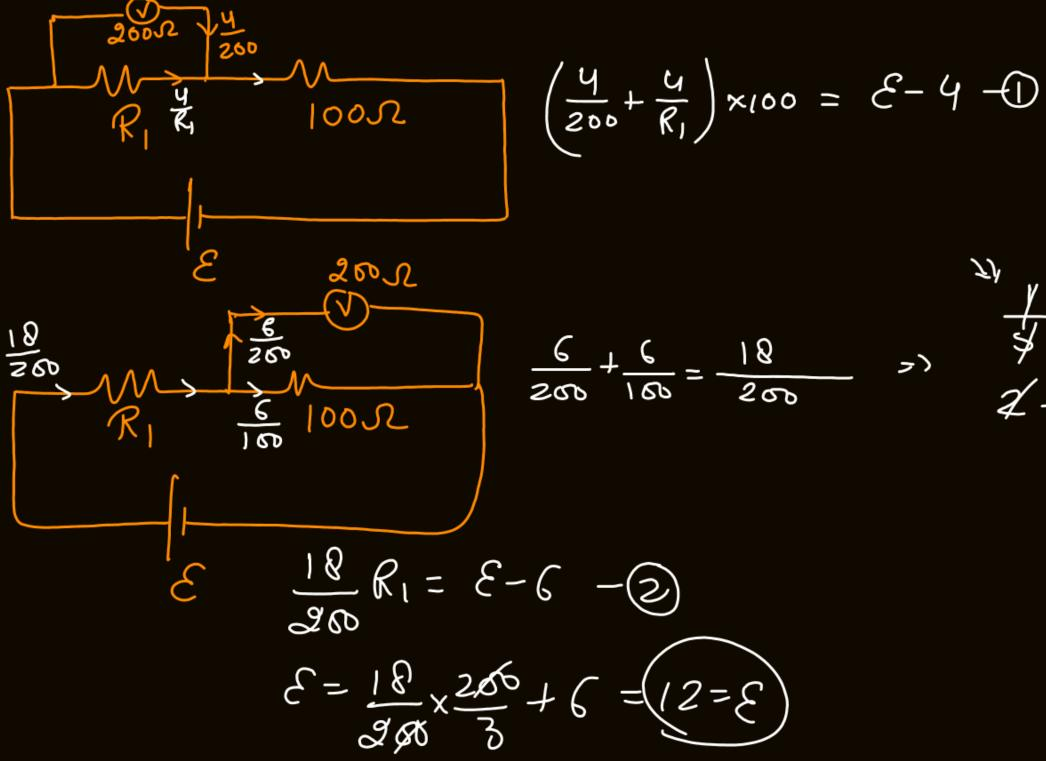
Q. 27: In the circuit shown in the Figure, cell is ideal and  $R_2 = 100 \ \Omega$ . A voltmeter of internal resistance  $200 \ \Omega$  reads  $V_{12} = 4 \ V$  and  $V_{23} = 6 \ V$  between the pair of points 1-2 and 2-3 respectively. What will be the reading of the voltmeter between the points 1-3.
