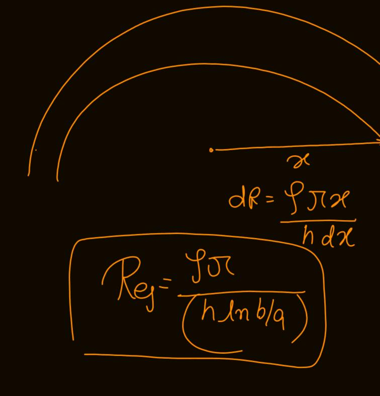
**Q. 50:** A conductor having resistivity  $\rho$  is bent in the shape of a half cylinder as shown in the figure. The inner and outer radii of the cylinder are a and b respectively and the height of the cylinder is h. A potential difference is applied across the two rectangular faces of the conductor. Calculate the resistance offered by the conductor.
